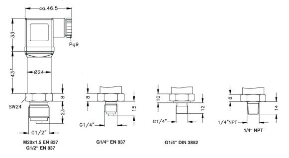
\* Pressure range PN = 40 MPa: total length increases by 12 mm
