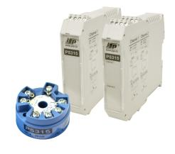
sensor. The inner sensor guarantees maximum accuracy and stability of cold junction temperature measurement of P5315 H10. For accurate measurement of thermocouples by transmitters P5315 Lxx for a DIN rail is needed to use setting for external compensation and use compensation terminal CTB3, respectively CTB4.
